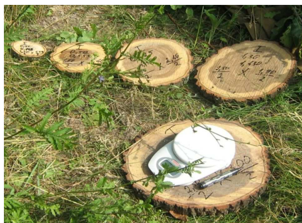
Figure 2. The test samples cut from the trunk of oak to determine density of biomass fractions
