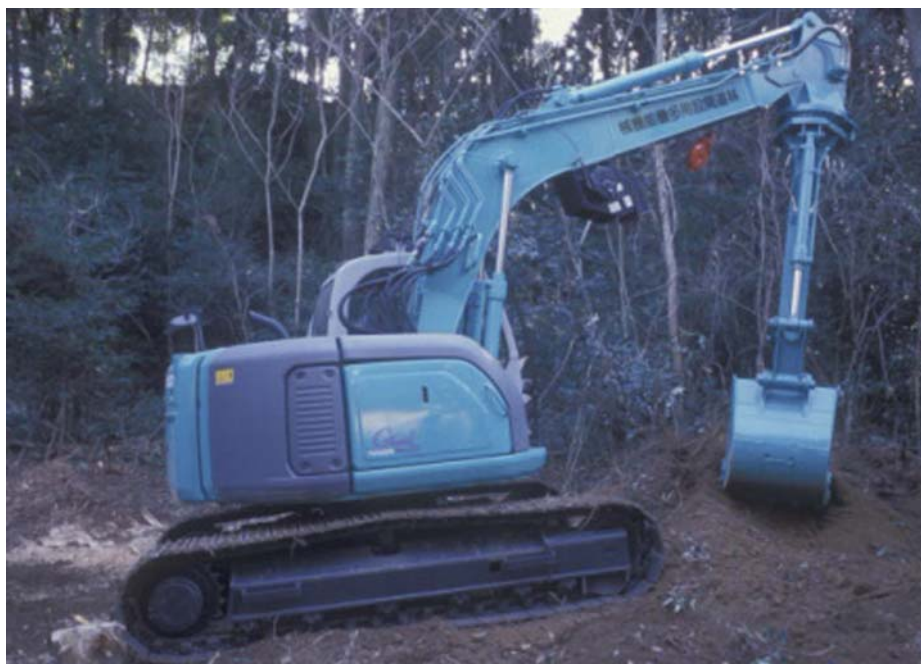
Figure 6. New excavator that can rotate its arm (2003) [2]
