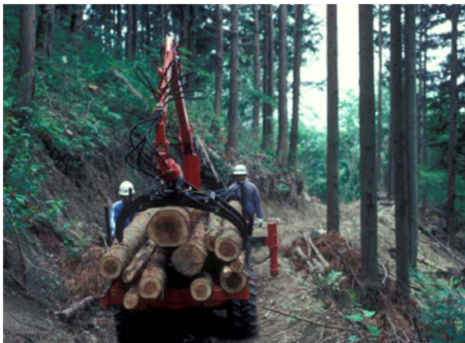
Figure 5. Mini-forwarder equipped with a grapple loader on an operation road 2.3 m in width (1987) [2]
