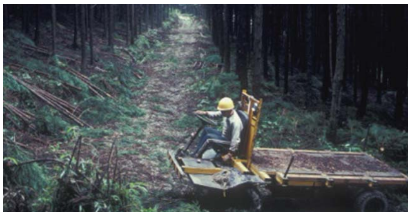
Figure 2. Prototype four wheeled forwarder on the operation road (1981) [2]
