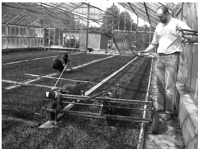
Figure 1. Sowing in the greenhouse; drilling section is mounted on the designed tool carrier
